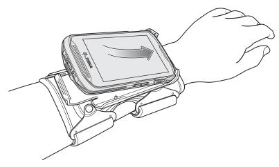
2. Rotate the bottom of the TC25 into the mount and snap into place.
