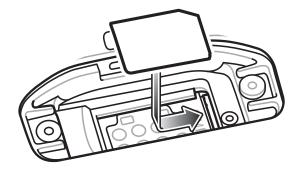
9. Push the SIM card in until it locks into the slot.
