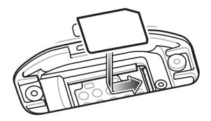
3. Push the SIM card in until it locks into the slot.
