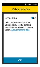
Touch **OK** to allow the TC25 to send analytics data. Touch the **Device Data** switch to disable the TC25 from sending analytics data and then **OK**.
