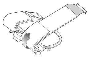
**4.** Feed the hard end through the slot in the front holder.
