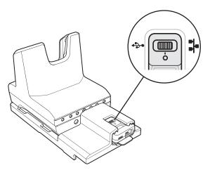
For Ethernet communication, slide the switch to the ## position.
