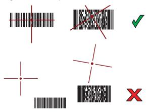
Figure 99 Pick List Mode with Multiple barcodes in Aiming Pattern
