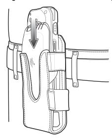
Insert the Trigger Handle into the holster with the device exit window facing down.
