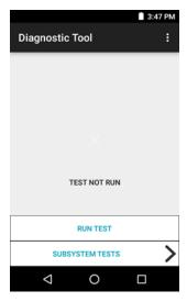
2. Touch **Run Test**. The app tests all enabled subsystems (by default only the Battery and System tests are enabled). See Settings on page 95 to enable subsystem tests.
