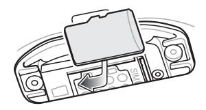
4. Push the microSD card into the SD card slot.
