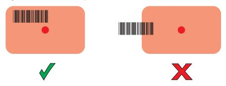
Figure 92 SE4710 Pick List Mode with Multiple Barcodes in Aiming Pattern
