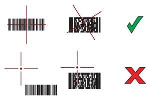
Figure 96 Pick List Mode with Multiple barcodes in Aiming Pattern
