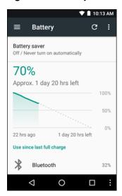
The **Battery** screen lists the applications using the battery. The discharge graph at the top of the screen shows the rate of the battery discharge since last charged (short periods of time when connected to a charger are shown as thin green lines at the bottom of the chart), and how long it has been running on battery power.
