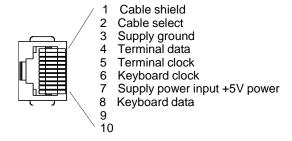
Note: Pin assignments are not compatible with legacy products. Use of a cable with improper pin assignments may lead to damage to the unit. Use of any cables not provided by the manufacturer may result in damage not covered by your warranty.
