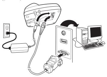
4. Plug the serial connector into the serial port on your computer. Tighten the two screws to secure the connector to the port.
