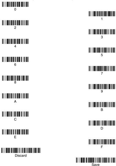
Note: If you make an error while scanning the letters or digits (before scanning Save), scan Discard, scan the correct letters or digits, and **Save**.
