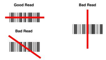
The best focus point for reading most code densities is about 5 inches (12.7 cm) from the unit. To read single or multiple symbols (on a page or on an object), hold the image scanner at an appropriate distance from the target, pull the trigger, and center the aiming line on the symbol.
