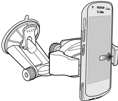
2. Rotate the other side of the device into the holder and gently release to collapse the holder and secure the device.
