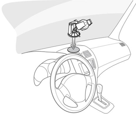
4. Push the lever towards the base to create a vacuum between the suction cup and the disc.
