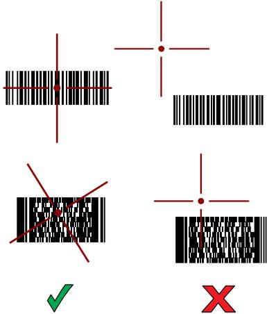
When the RS507/RS507X is in Pick List mode, the RS507/RS507X does not decode the barcode until the center of the crosshair touches the barcode.
