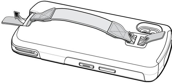
2. Pull the ends of the hand strap through the slots.
