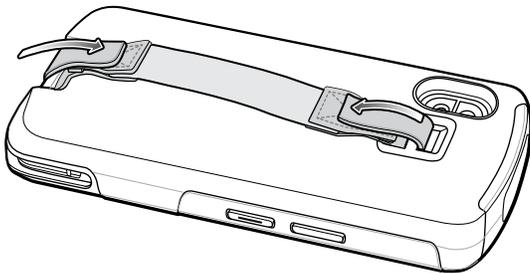
4. Place hand between device and hand strap and adjust hand strap as necessary.
