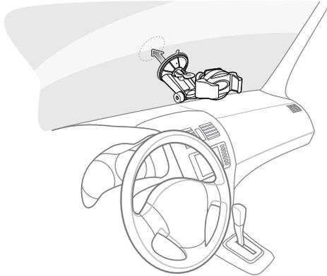
2. Push the lever towards the base to create a vacuum between the suction cup and the windshield.
