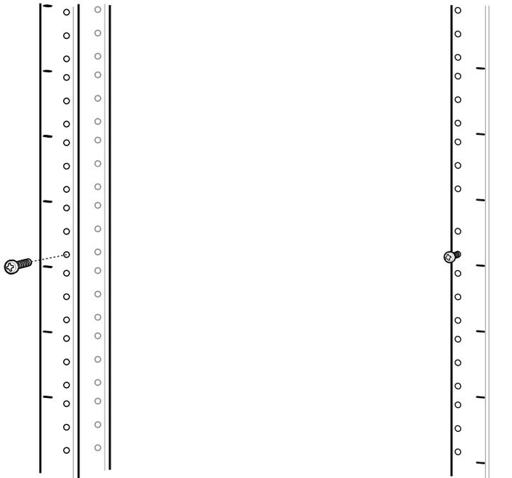
3. Align the mounting bracket's top mounting key holes with the screws.
