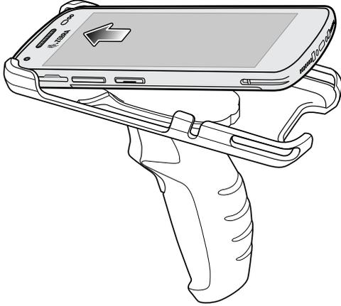
2. Rotate the device down and press down until it snaps into place.
