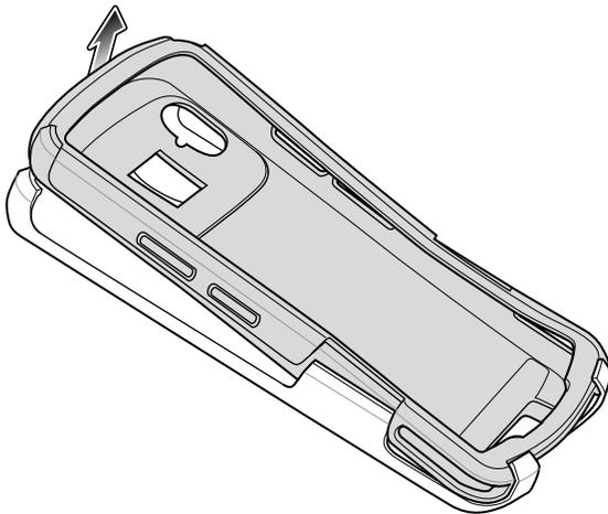
2. Insert the bottom of the device into the bottom of the boot.
