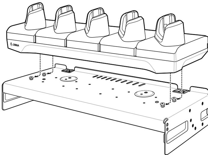
8. Secure cradle to top tray with two M2.5 safety screws.
