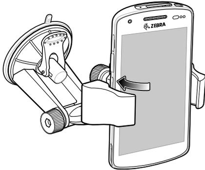
3. Loosen the mount and holder knobs and adjust the device for best viewing.
