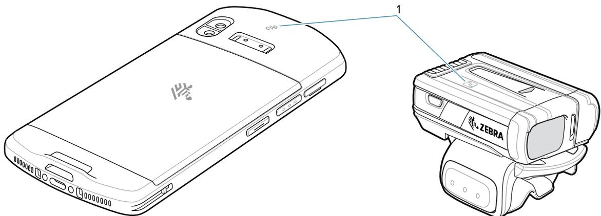
The Status LED blinks blue indicating that the Ring Scanner is attempting to establish a connection with the device. When a connection is established, the Status LED turns off and the Ring Scanner emits a single string of low/high beeps.
