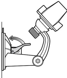
3. Make sure that the suction bond is strong enough before installing the device.
