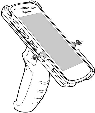
2. Rotate the bottom of the device up.
