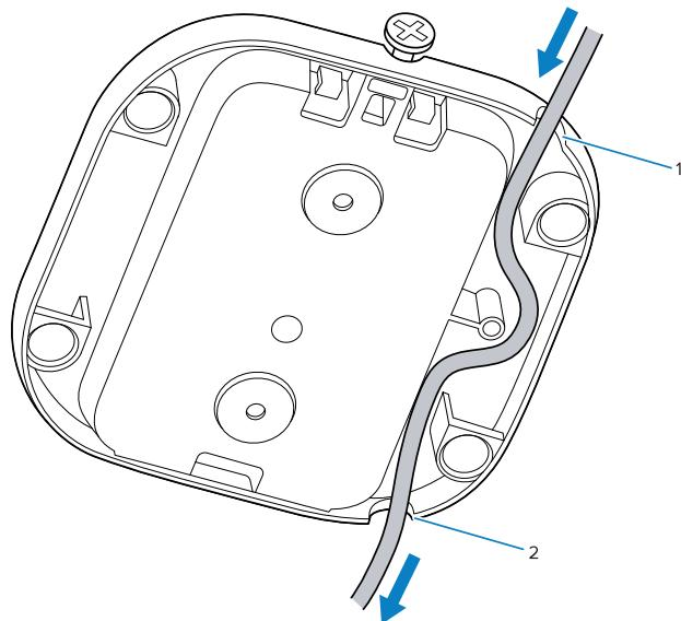
**4.** With the cable installed, hold the wide base to the predetermined location on the wall, and then insert and tighten #6 wood screws (not provided) through each screw hole in the wide base.
