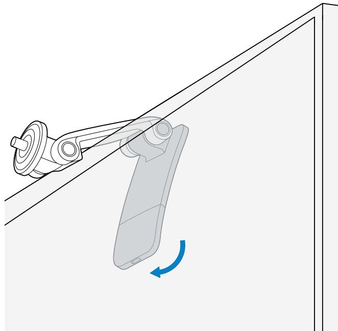
5. Mount the scanner onto the top swivel plate, and then orient the scanner window to face down as needed.
