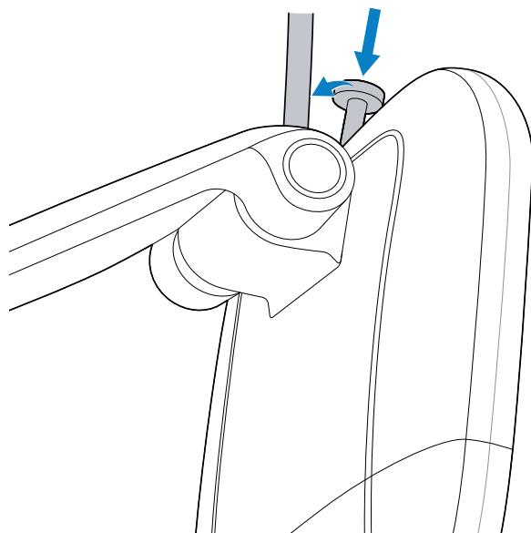
7. Connect the power cable to the scanner, and then mount the scanner onto the top swivel plate.
