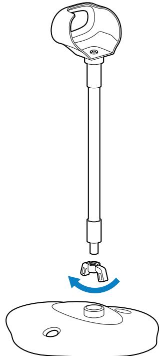
2. Insert the threaded end of the gooseneck into the base.
