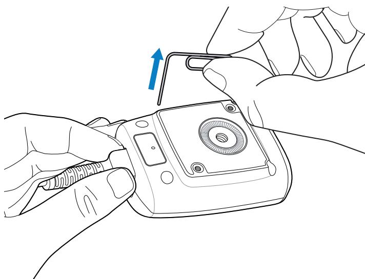
6. Fully remove the cable.
