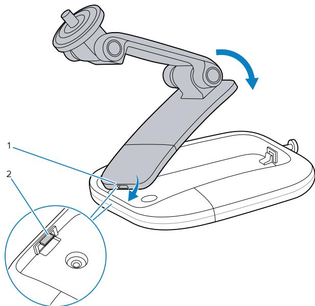
6. Using a Philips-head screwdriver, tighten the wide base screw to fasten the narrow base to the wide base.
