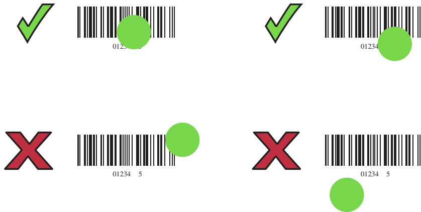
The aiming dot is smaller when the scanner is closer to the barcode and larger when it is farther away. Scan barcodes with smaller bars or elements closer to the scanner and those with larger bars or elements farther from the scanner.
