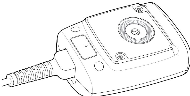
2. Grasp the strain relief section of the cable with your fingers pressed against the device.
