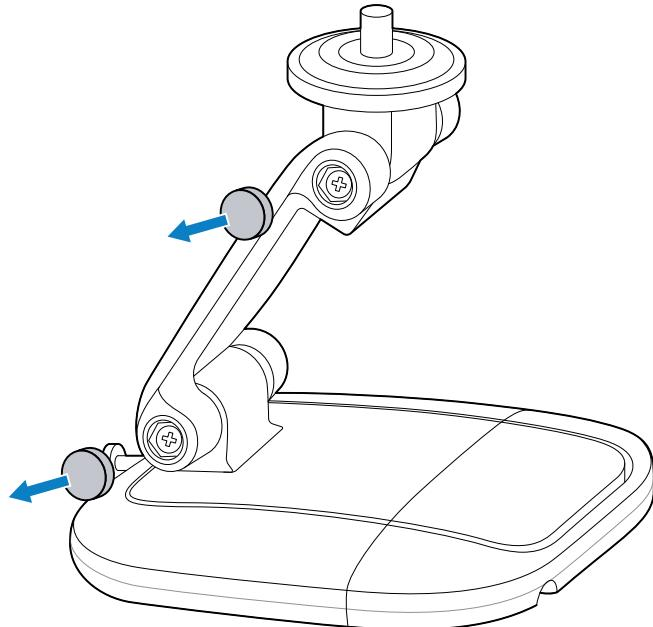
2. Using a Philips-head screwdriver, adjust the tightness of the pivot joint as needed, and then reinsert the rubber plug into the pivot joint.
