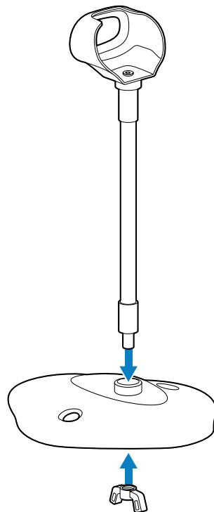
3. From the underside of the base, fasten the gooseneck by screwing and tightening the wingnut into it.
