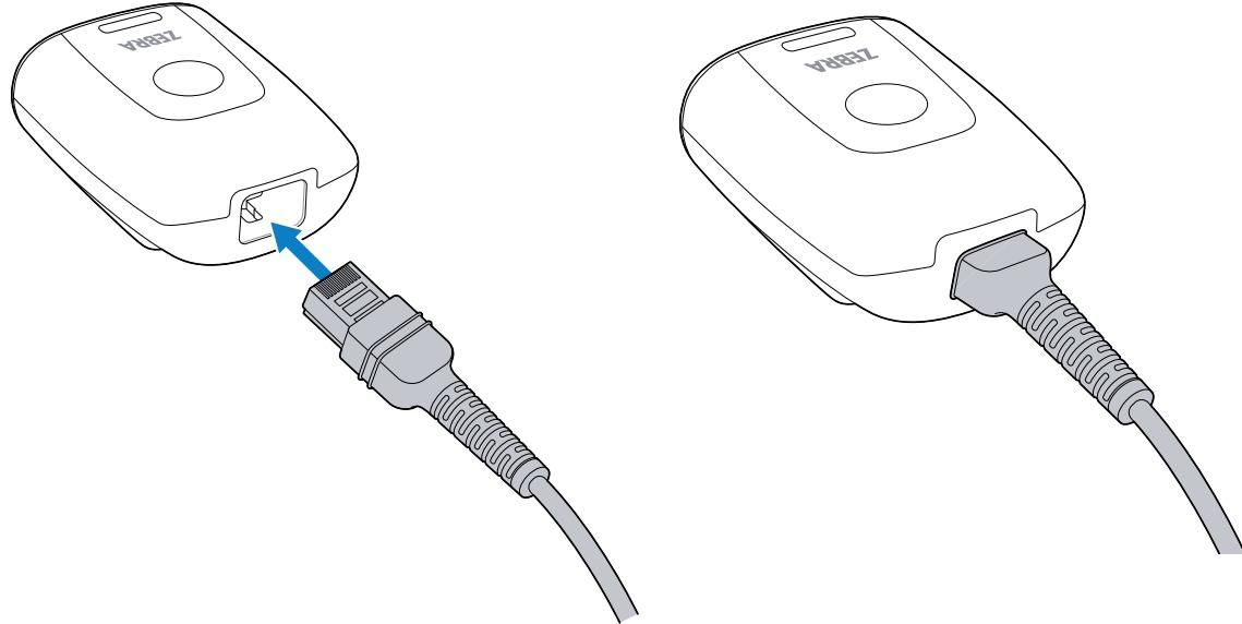
2. Connect the other end of the cable to either the USB or RS-232 port on your host computer. For more information, go to [USB Interface Connection](#) on page 91 or [Connecting an RS-232 Interface](#) on page 108.
