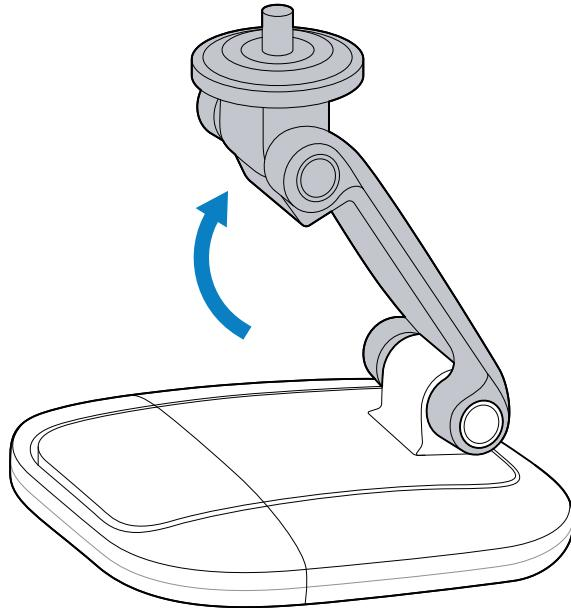
3. Mount the scanner onto the top swivel plate, and then orient the scanner window to face down as needed.
