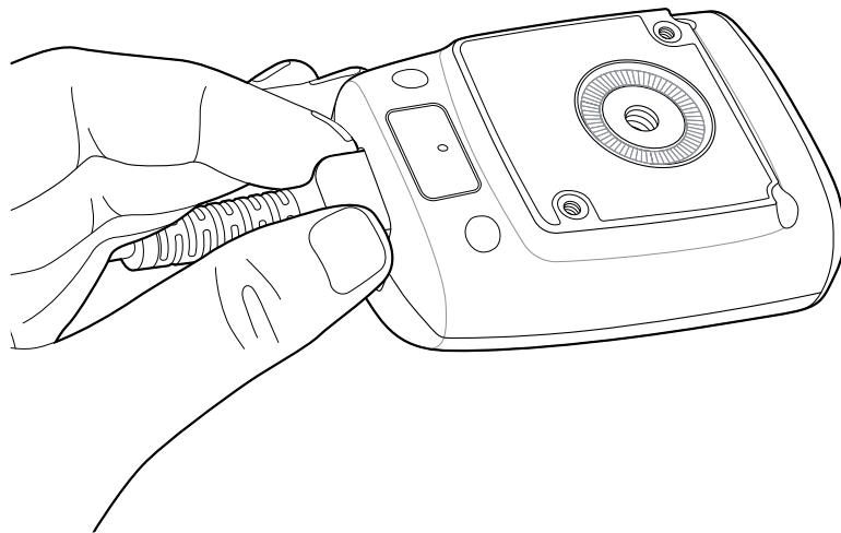
3. With your other hand, insert a paper clip into the pinhole to push down the cable latch.
