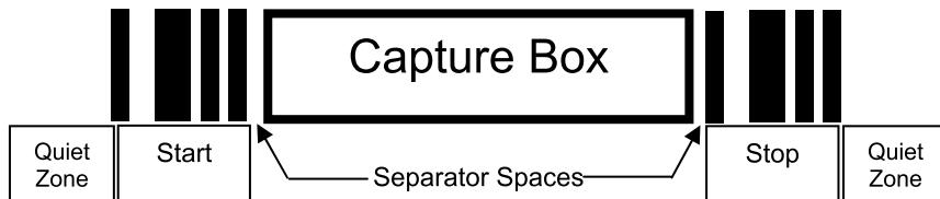
The separator spaces on either side of the signature capture box can be between 1X and 3X wide.
