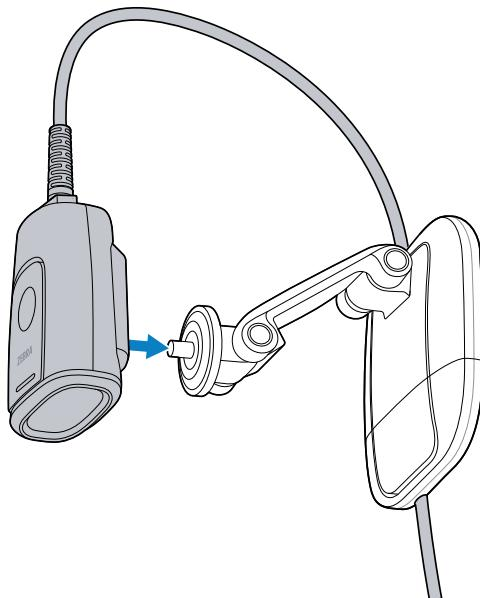
8. Orient the scanner window to face down as needed.
